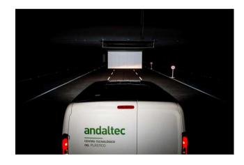
ANDALTEC PHOTOMETRIC TUNNEL HAS THE FOLLOWING DIMENSIONS: 80m LONG X 20m WIDE. THIS IS THE LARGEST PHOTOMETRIC TUNNEL IN SPAIN AND ONE OF THE LARGEST IN EUROPE.
